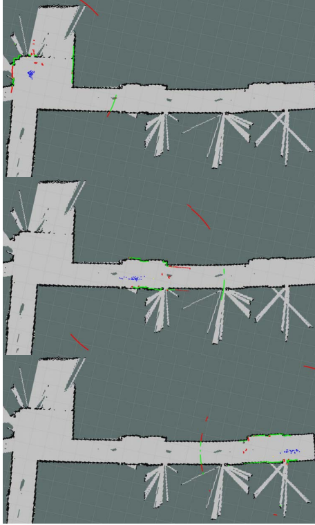
Fig. 18. The 100 positions after different relocalization and resampling
