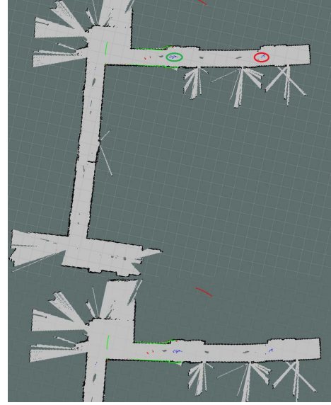
Fig. 16. The 100 positions after a first relocalization and resampling. In the bottom part, we see the best position and its matching with the grid map
