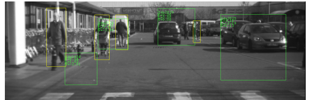
Fig. 4. Outputs from the post processing modules: (a) green bounding boxes represent the detected vehicles; (b) yellow bounding boxes represent the pedestrians detected by the pedestrian detector.
