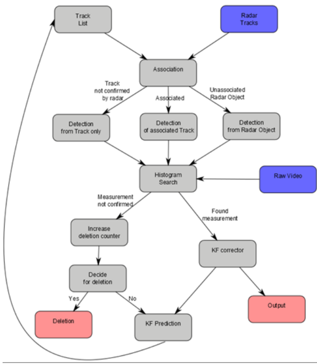
Fig. 3. Pedestrian Detector work flow. Inputs are depicted in blue and outputs in red.
