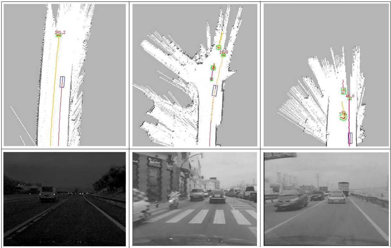
Fig. 7. Experimental results show that our algorithm can successfully perform both SLAM and DATMO in real time for different environments
