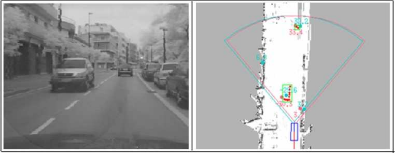
Fig. 6. Moving object detected from laser data is confirmed by radar data.
