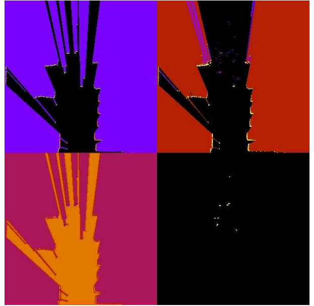
Fig. 9 Upper left: the observed map \mathcal{M}_o . Upper right: the static map \mathcal{M}_s . Bottom left: the difference map \mathcal{M}_d . Bottom right: the extracted foreground. For all the maps, the more hot is the color, the more positive is the value.
