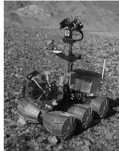
Figure 9: The Marsokhod rover
